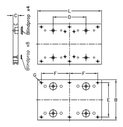
$\begin{array}{lll} B & = 185 \\ C & = 20.00 \\ d & = 198 \\ E & = 160 \\ F & = 270 \\ For bearing = 54 \\ For slide & = L/NL 76 \\ L & = 300 \\ \end{array}$
